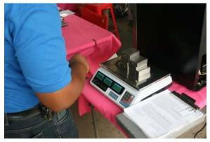
Figure 1. During the inspection process, TDA WM staff use certified weight sets to test the scale's accuracy.
