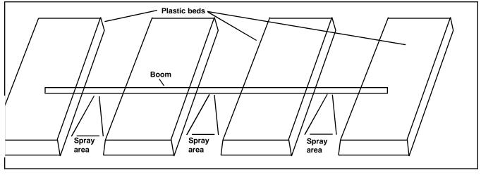
Figure 4. Illustration of a directed spray for weed control when cataloupes are being produced on plastic.
