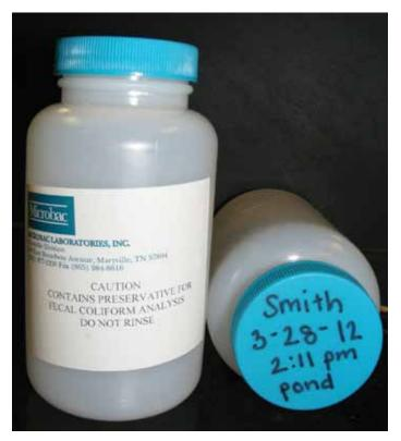
Figure 2. Sampling bottle properly labeled with name, date, time and type of water source.
