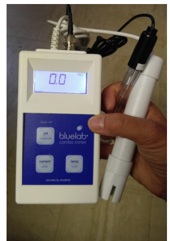
Figure 5. These are small handheld pH and EC meters that can be a useful addition to a hydroponic growing system.
