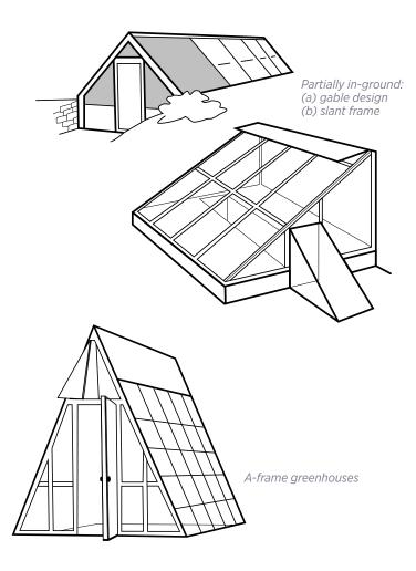
FIGURE 3. Examples of different designs for small greenhouses
