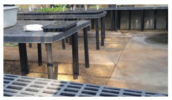
FIGURE 4. A small greenhouse with concrete walkways and gravel under the benches to support drainage.
