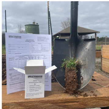
(Soil sample test box and submission form with an example of a pulled core subsample-photo J. Stefanski)
